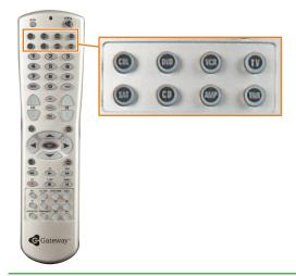
Programs the remote control to recognize a component. For programming instructions, see "Programming the remote control" on page 7.
